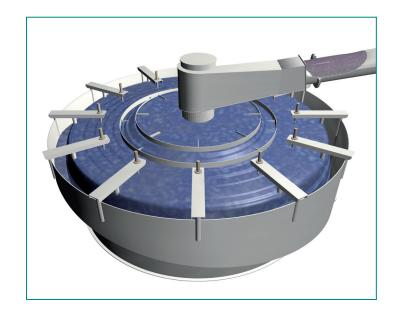
The allflux® separator uses fluidized bed technology for the separation and hydraulic classification of slurried fines. The two-step process permits the handling of slurries without pre-thickening. The coarse and heavy particles are separated in the coarse section.
