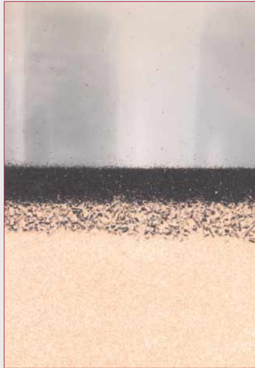
Fig. 3: Organic Impurities on Top of the Autogenous Fluidized Bed in a Sand Cleaning Application.
