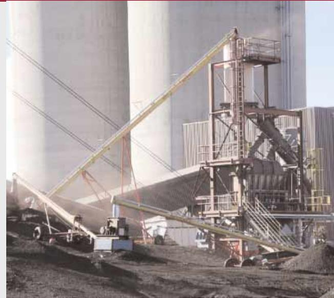
Figure 4. | Module 5: Pilot Dryer and Dried coal storage trailer
